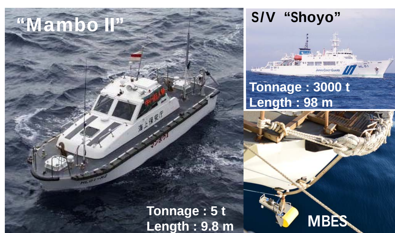
Fig. 10 Autonomous survey boat "Manbo II" (left), her mother vessel "Shoyo" (upper right), and a MBES (R2sonic2022) mounted on the Manbo II (lower right). Manbo II was designed for survey of active submarine volcanoes and was commissioned in 1998.
