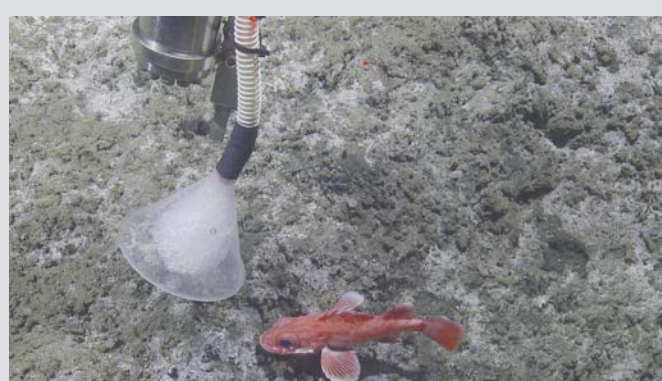
Figure 3 (above): ROV Hercules gathers seep bubbles with a funnel to collect in a gas tight chamber for gas composition analysis.
